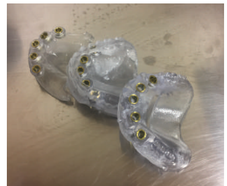
Full Arch surgical guides printed from MED610
