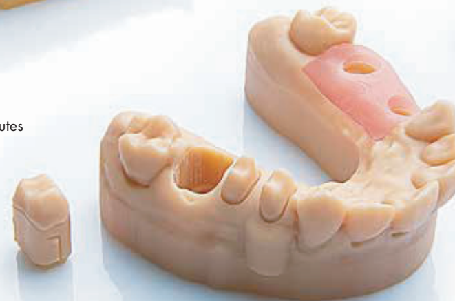
28x gingiva mask units, printed in ~ 15 minutes
