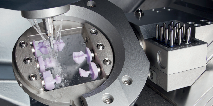
The R5 swivels the spindle (B axis) by up to ±35°. This means that the workpiece holder only needs one moving axis (A axis) and the entire system gains stability.
