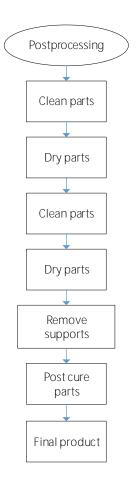
Cleaning in 2-propanol (min. >96 %) (max. 5 minutes); Cleaning under pouring conditions (no ultrasonic); Recommendation: Magnetic stirrer with bar or lab shaker. Clean and rinse gaps separately.
